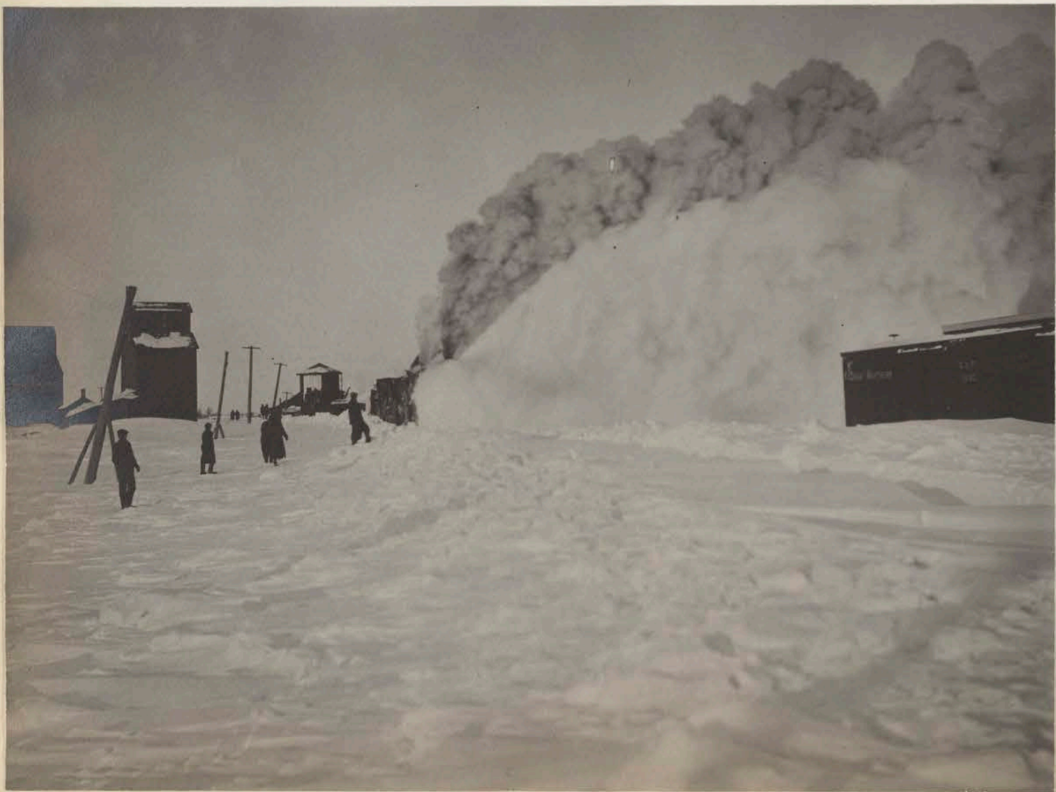
250 Action of rotary snow plow, near Langdon N.D. winter of 1906. In February the snow had drifted in places as quite to over- top the coaches of the trains.
